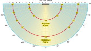
Measured at 2 watts setting in anechoic chamber
